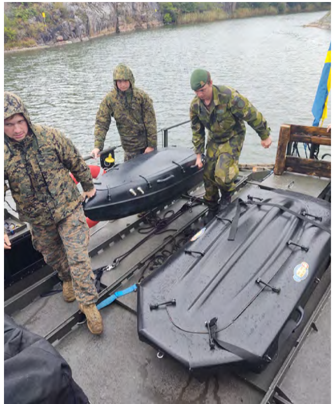
"US and Swedish marines recover an AMY unmanned surface vehicle (an ONR-supported technology) aboard a Combat Boat 90, a small high-performance light craft of Swedish manufacture. To the right is the larger Reckless unmanned surface vehicle, which is being used for logistics support of small units in austere littoral environments. Photo by Edward Lundquist
