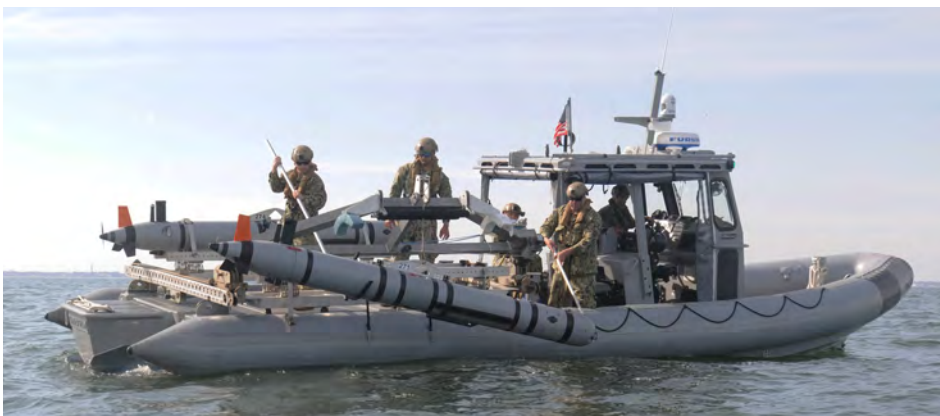
The MK-18 Mod 2 Kingsfish, now a standard unmanned underwater vehicle used by mobile diving and salvage, explosive ordnance disposal, and mine countermeasures units, is a modified version of the REMUS unmanned vehicle originally developed by Woods Hole Oceanographic Institution with the support of the Office of Naval Research. The first major use of this technology occurred in 2003 with the clearing of Iraqi ports in the aftermath of Operation Iraqi Freedom. Photo by MC2 Benjamin Woody
