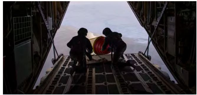
An air-deployable expendable ice buoy is deployed in the high Arctic near the North Pole from a Royal Danish Air Force C-130 aircraft operating out of Thule Air Force Base in Greenland, as part of the International Arctic Buoy Program. Photo by John F. Williams
